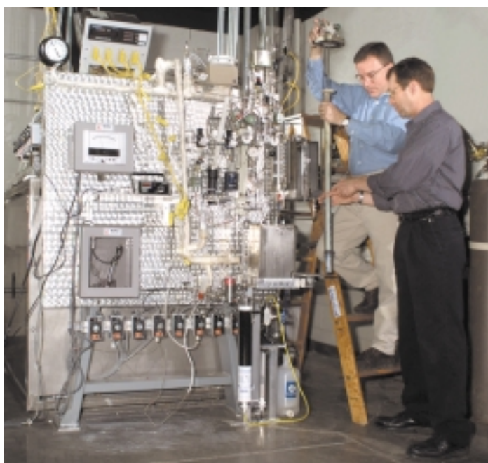
The Keiser rig, a facility developed at ORNL, was used to evaluate how combustor liner materials and coatings would react under exposure to combustion gases in gas turbines.
