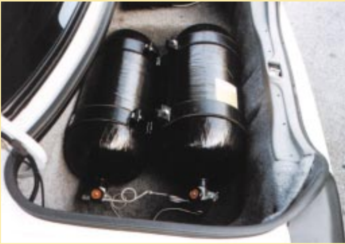
Composite CNG tanks mounted inside an automobile trunk (Photo courtesy of Lincoln Composites).
