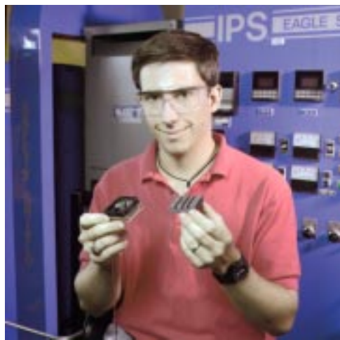
James Klett holds a heat exchanger and heat sink for power electronics formed from carbon foam. They can be much smaller and lighter than conventional aluminum heat transfer devices.
