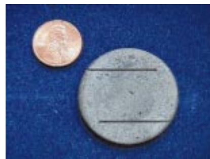
The bipolar plate (right) showing gas channels
