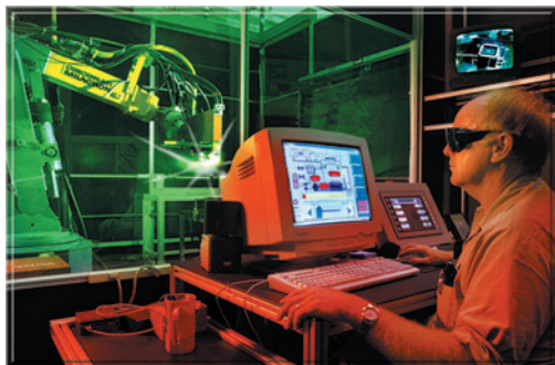
Plasma arc lamp in operation in ORNL's Infrared Processing Center.
