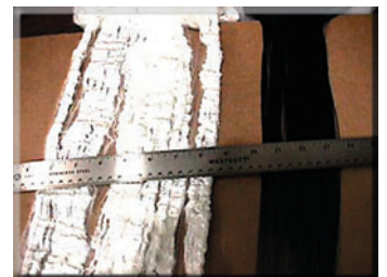
Textile-grade PAN before (left) and after being converted to carbon fiber.
