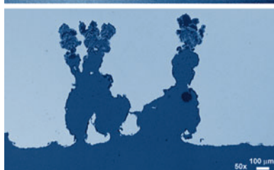
Surface cracking on boiler tube interior (top) and metallograph showing its penetration of the tube wall.
