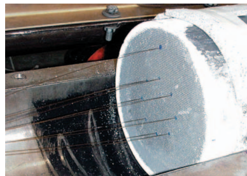
Capillaries inserted in a catalyst for SpaciMS measurement.
