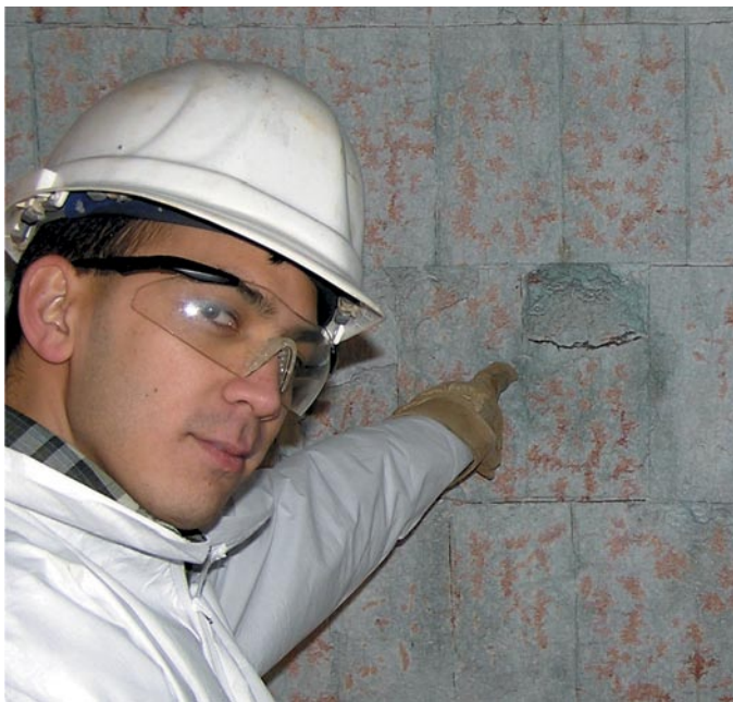
ORNL's James Hemrick points out a test brick in the refractory lining of the black liquor gasifier at the New Bern paper mill.
