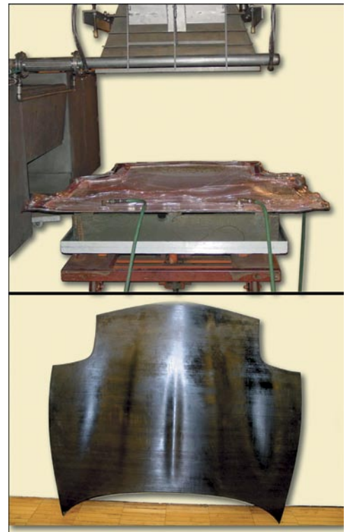
PMC outer hood ready for e-beam curing (top). Finished PMC outer hood (bottom).
