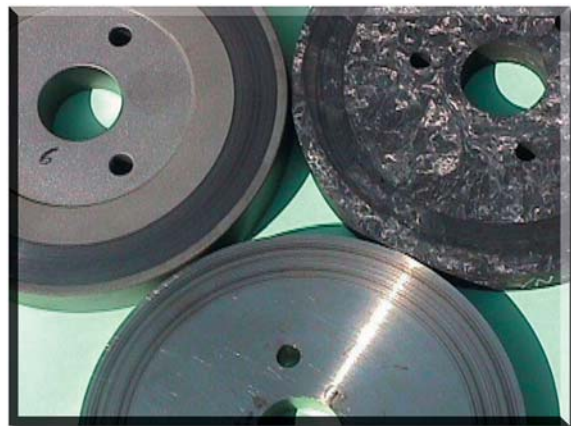
Potential brake disc materials: commercially coated Ti (upper left), experimental ceramic composite (upper right), and uncoated Ti alloy (bottom).
