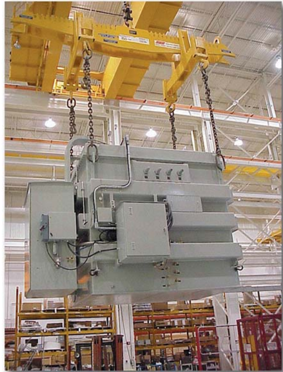
Moving the 5/10-MVA transformer to the Waukesha Electric Systems test area.
