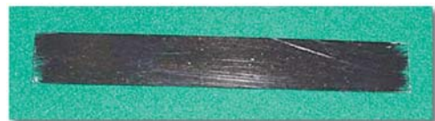
Small composite piece prepared from lignin-based carbon fiber.
