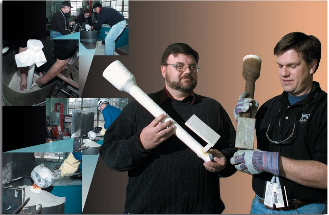
Preparing to cast an aluminum part by lost-foam casting (left, top down): securing the EPS mold in sand, pouring molten metal into the mold. At right, Ralph Dinwiddie of ORNL with an EPS mold and Dennis Nolan of FOSECO-Morval with a cast aluminum part.
