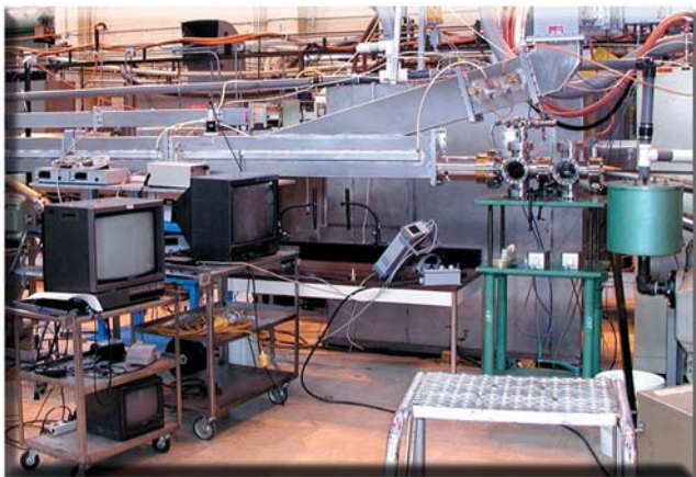
ORNL's microwave-assisted processing line has attained a speed of 200 inches per minute.
