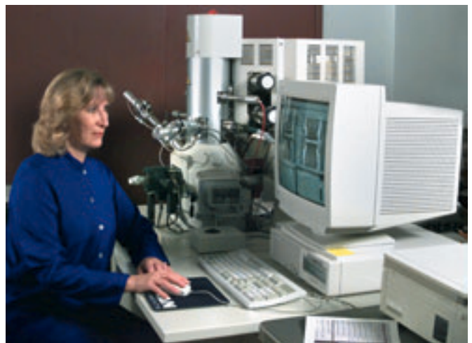
ORNL researcher Dorothy Coffey uses the focused ion beam milling instrument in the HTML.
