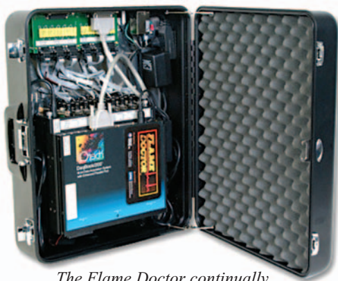
The Flame Doctor continually analyzes the combustion quality of individual coal burners.
