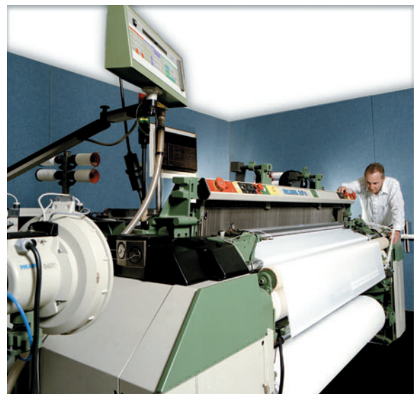
This on-line defect sensor inspects fabric for flaws as it is woven, saving time and avoiding waste.
