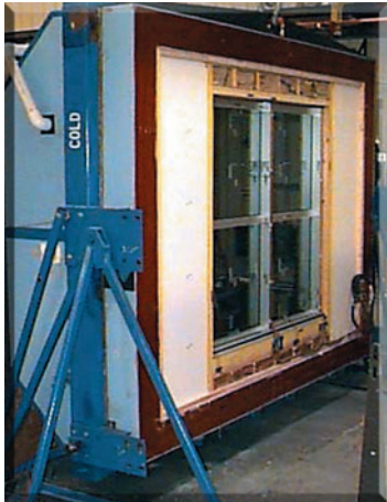
A wall assembly being tested at ORNL. Data from such research are used in the energy efficiency calculators.
