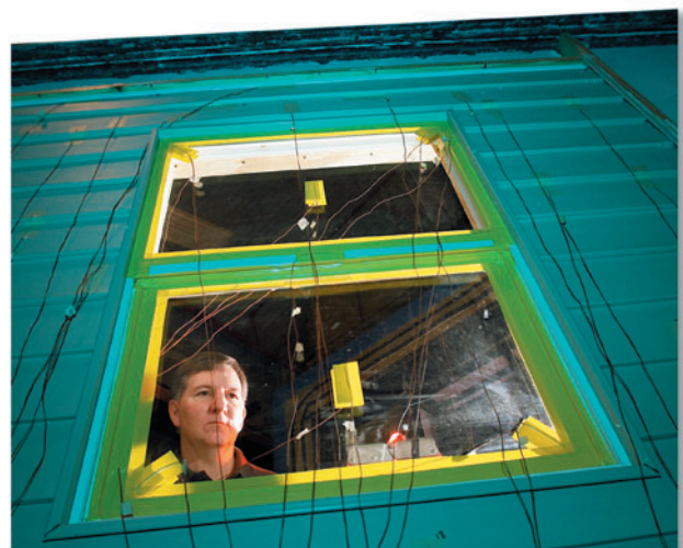
Phil Childs of ORNL's Buildings Technology Center monitors the energy efficiency of a wall system and window.
