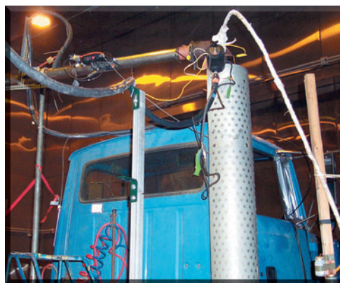
Instrumented tractor rig in the environmental chamber at the Aberdeen Test Center.
