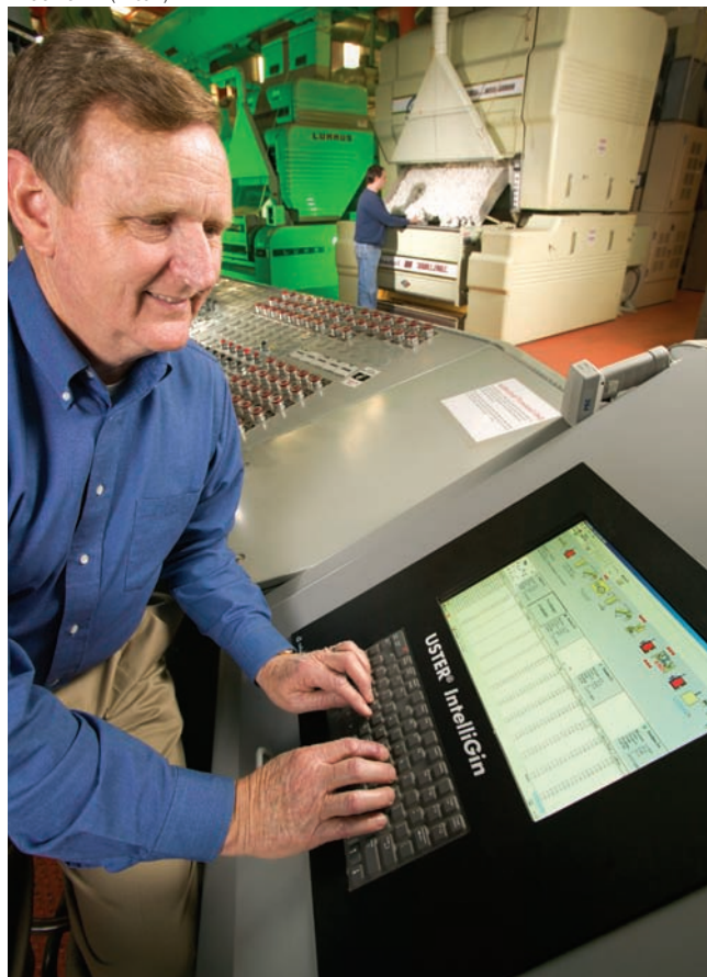
W. Stanley Anthony inputs control data into a computerized process control system he developed with agricultural engineer Richard Byler. In the background cotton ginner J. Kim Sabbatini inspects cotton at a gin stand. The control system is marketed under the trade name “IntelliGin.”
