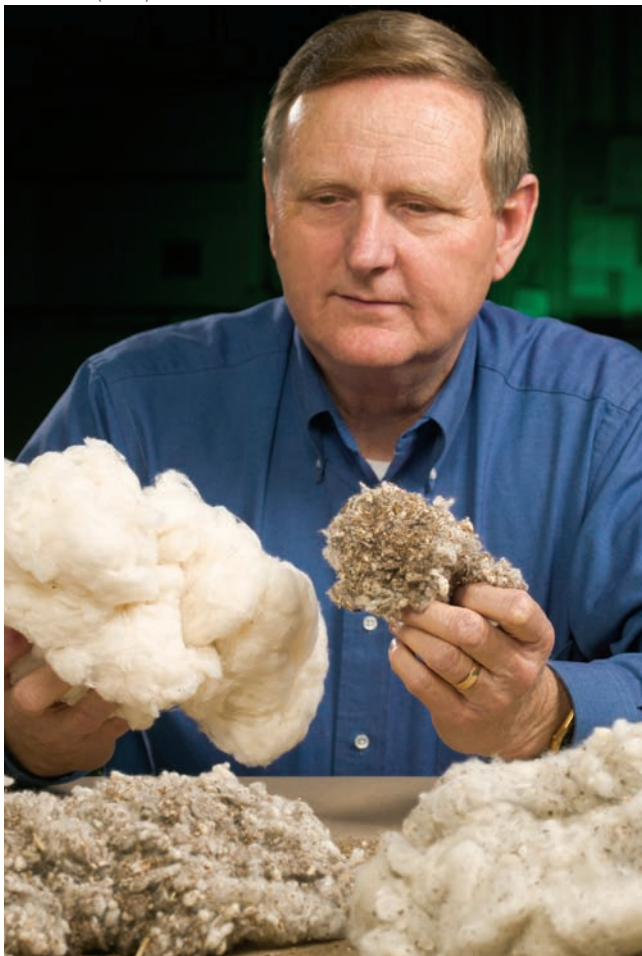
Agricultural engineer W. Stanley Anthony examines samples of lint and foreign matter and clean cotton fiber that was processed with a new saw-type lint cleaner he developed, marketed under the trade name “LouverMax.”
