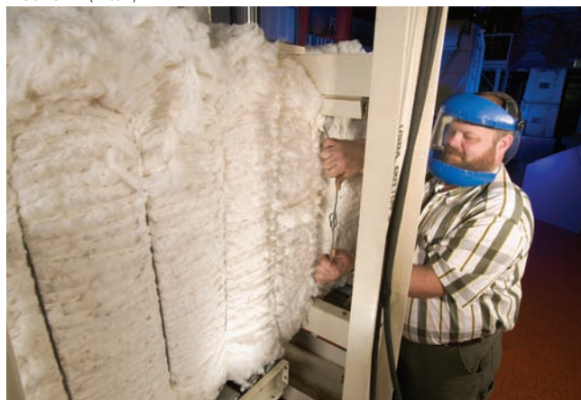
Tony Deerman, machinist, replaces a broken bale tie on a cotton bale using a device patented by Anthony and marketed commercially under the trade name “Ultrabander.” Deerman constructed this prototype.
