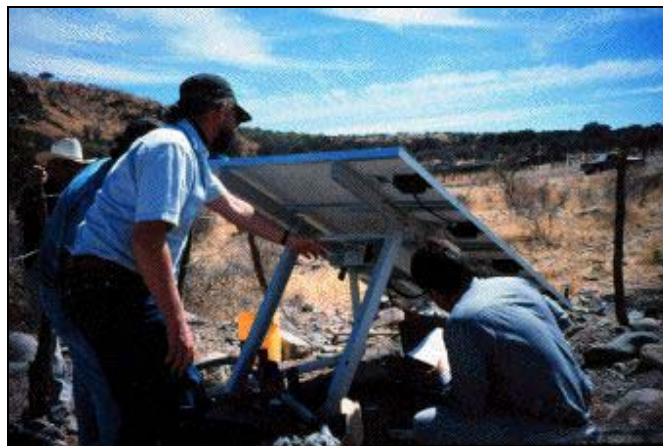
Figure 7-6. Chihuahuan agricultural engineers learning how to conduct an acceptance test on a PV water pumping system.
