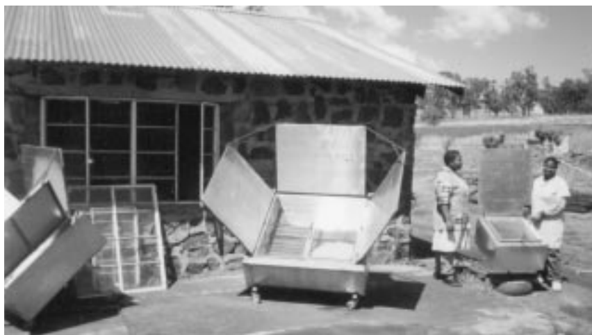
Figure 2.5. Solar ovens—household model on right.
