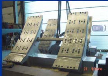
Modules in the region of the saddles simply rest on swivel bolts which are mounted in the holes shown.
