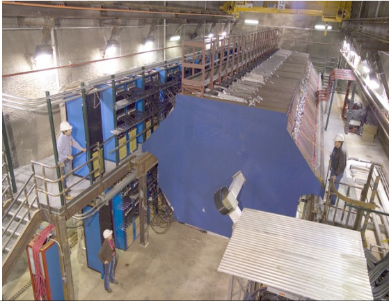
MINOS Near Detector at Fermilab: ANL built all Near Detector scintillator modules, and all its readout electronics
