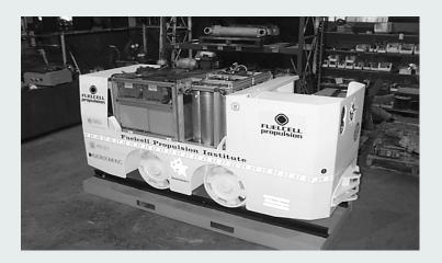
Fuel cells can give mining locomotives such as the one above the mobility and energy capacity of a diesel vehicle but the environmental characteristics of electric vehicles.
