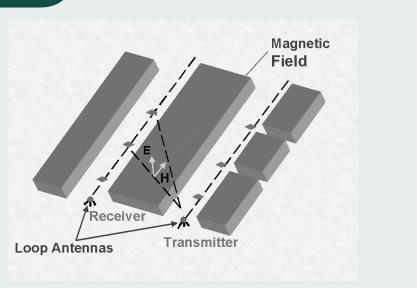
RIM transmits electromagnetic waves on one side of the geologic target and uses a receiver on the other side to collect data about the geologic mass.
