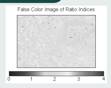
The dark areas above show false coloring used to highlight the presence of sulfides within the ore.
