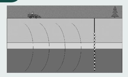
Above illustration shows seismic sensors in dry a vertical borehole for surface mining/quarrying.
