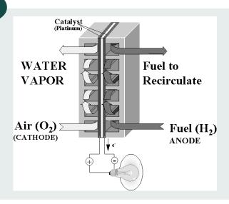
Fuel cells use hydrogen and oxygen to produce electrical energy with water as the only by-product.
