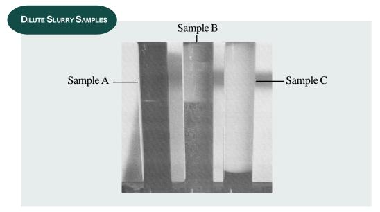
Selective flocculation may be used to separate two or more finely divided minerals in a dilute slurry. With appropriate reagents under the right conditions in the dispersed slurry (sample A), one of the constituents flocculates (dark aggregates in the bottom of sample B) and settles or is otherwise separated from the unflocculated constituents that remain in suspension (sample C).
