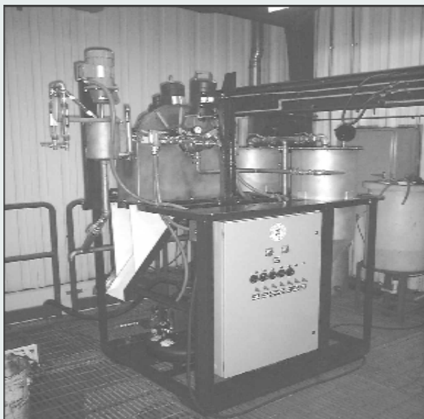
Pilot-scale disc filter used for dewatering tests.
