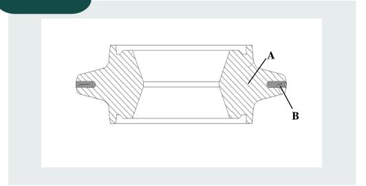
The disc cutter body material (A) surrounding a hard material insert (B) will be HIPped in one step by the CastCon Process.
