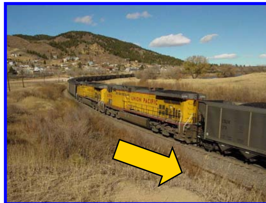
2 Distributed Power units at mid-train (unmanned)
