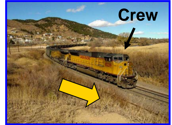
2 primary units on head-end of train (lead unit manned)
