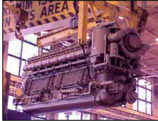
Typical Loco. diesel engine ... 1500-to-4400 HP 125-367 HP/cylinder
