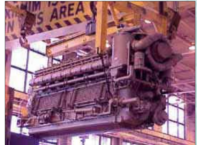
Typical 4400 hp locomotive diesel engine ... weighs 46,000 pounds
