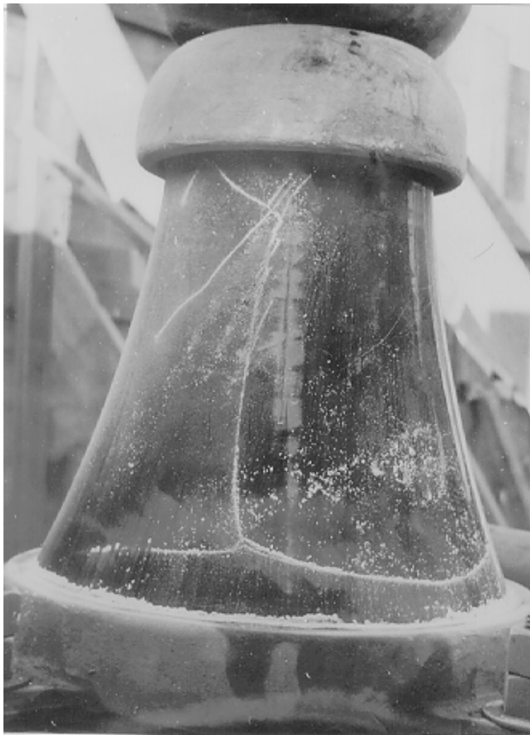
Figure E-24 Results of Statifluxing a Base Insulator. The powder indicates cracks not otherwise visible.
