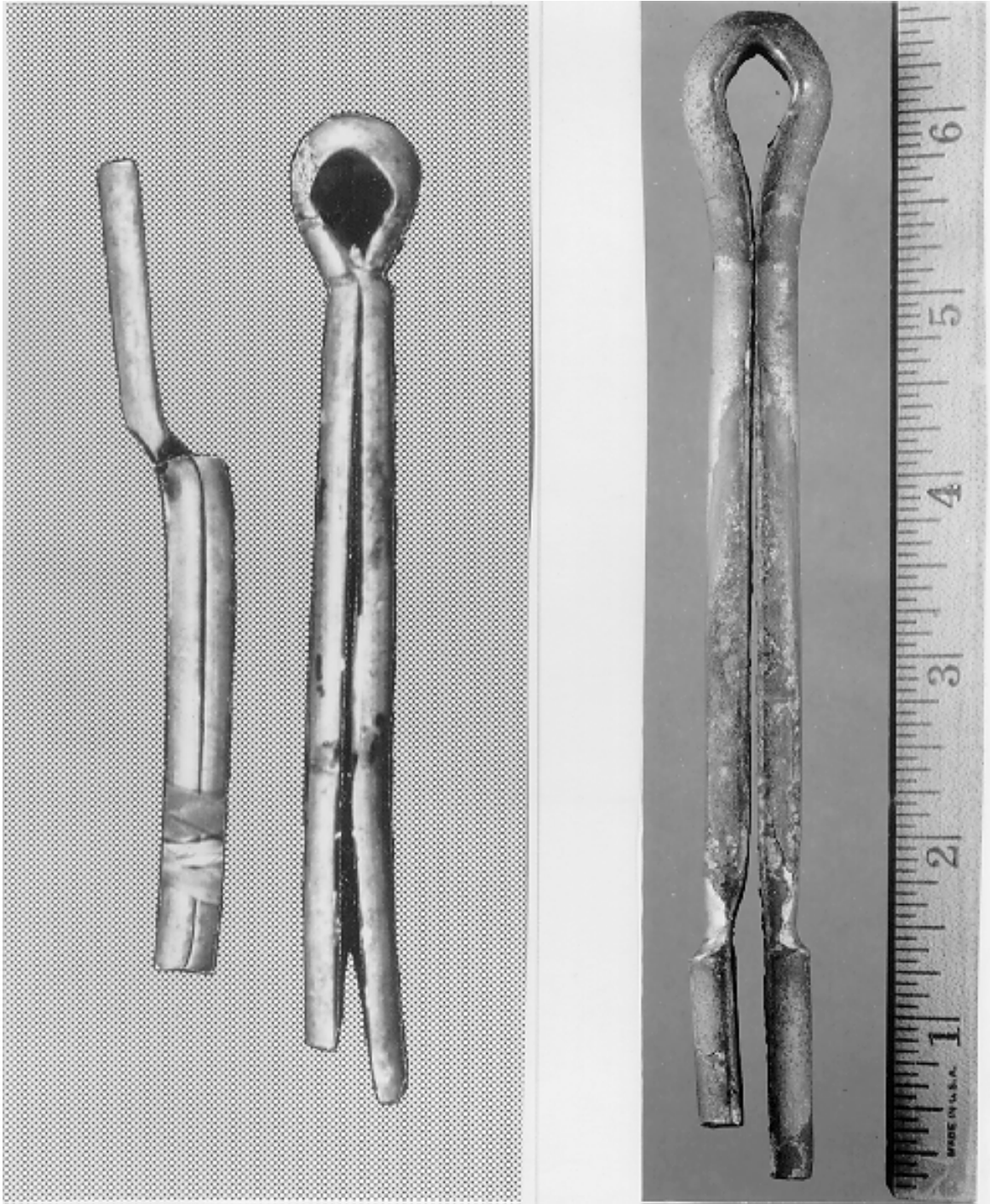
Figure 6-7 Wear of cotter pins.
