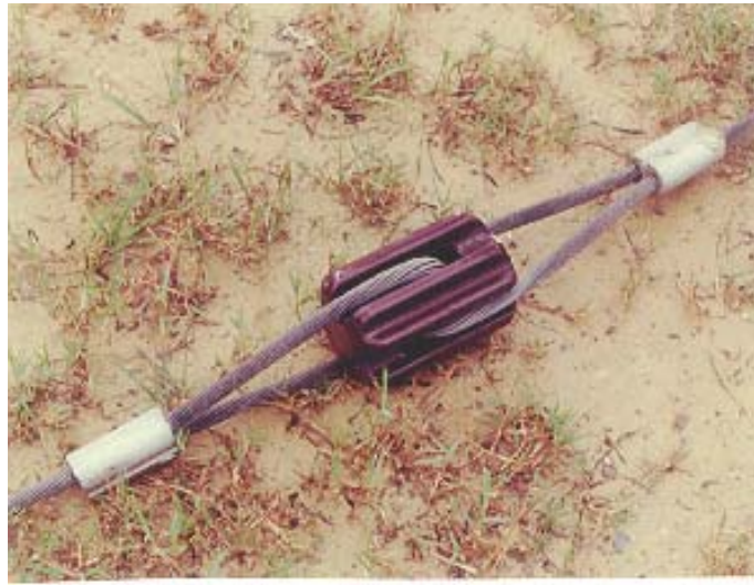
Figure 6-8b Closed end johnny ball insulator.
