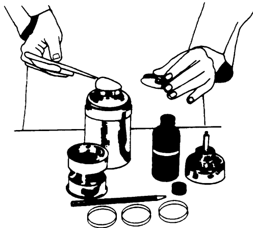
Figure 3-G Removing the membrane filter from the filter holder
