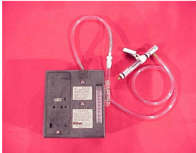
Figure 9-2. Sorbent Tube Sampling Train (Gilian Pump)
