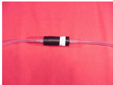
Figure 4-4c. Asbestos Cassette in-line
