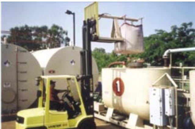
Figure 41—Dry powder mixing operation batch mixer (Redding, CA).
