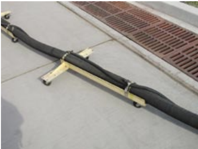
Figure 60—Loading hose and hose skates (San Bernardino, CA).
