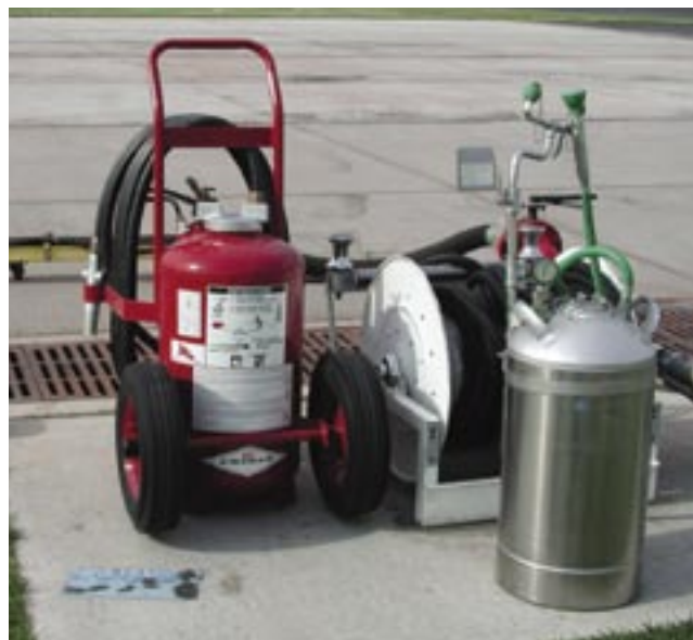
Figure 19—Fire extinguisher and portable eyewash (San Bernardino, CA).
