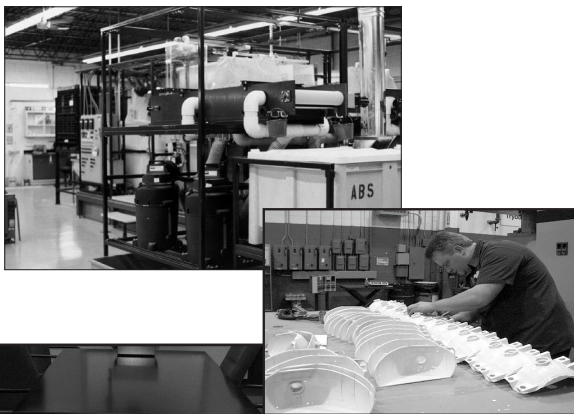
Argonne's froth flotation technology results in a high-quality ABS material that can be used to manufacture products such as the automotive lighting parts shown at right.
