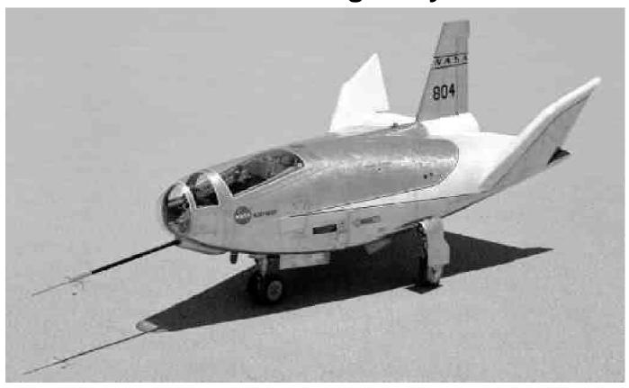
The HL-10 was one of five lifting body designs flown at NASA's Dryden Flight Research Center, Edwards, Calif., from July 1966 to November 1975 to study and validate the concept of safely maneuvering and landing a low lift-over-drag vehicle designed for reentry from space. It is now on permanent public display near the main entrance of Dryden.
