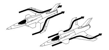
Reverse airflow—forward-swept wing vs. aft swept wing. On the forward-swept wing, ailerons remained unstalled at high angles of attack because the air over the forward swept wing tended to flow inward toward the root of the wing rather than outward toward the wing tip as on an aft-swept wing. This provided better airflow over the ailerons and prevented stalling (loss of lift) at high angles of attack.
