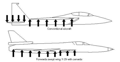
X-29 - designed with relaxed static stability to achieve less drag, more maneuverability, increased fuel efficiency. Arrows in upper illustration indicate drag-producing opposing downward forces on rear stabilizers to achieve stability. X-29 canards share lifting loads, reducing drag.
