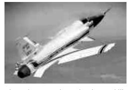
movable canards, enhanced maneuvering and cruise capabilities at transonic speeds. That phase was flown with the No. 1 X-29 aircraft and ended in 1989. NASA's high-angle-of-attack research program with X-29 No. 2 ended in 1991 and demonstrated that the aircraft design had better-than-expected control and maneuverability at angles of attack up to 45 degrees.
