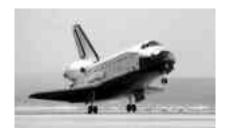
The prototype orbiter Enterprise was used in ALT to verify the glide and handling qualities of the vehicle following its return into the atmosphere from space. During ALT, Enterprise was taken aloft on the NASA 747 Shuttle Carrier Aircraft and air
