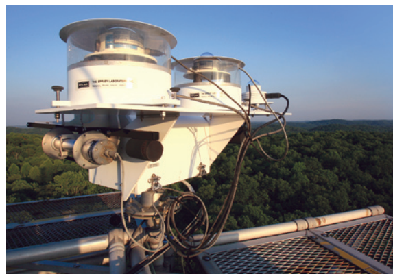
A radiometer atop the Walker Branch Watershed tower measures radiation from the sun and sky.
