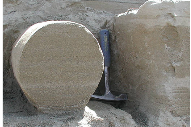
Core dissection shows that sorbed Sr 2+ is associated with dry, sandy sediments.
