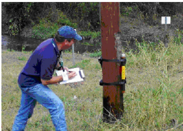
Pressure sensor strapped to a power pole near Vinton, Louisiana.
