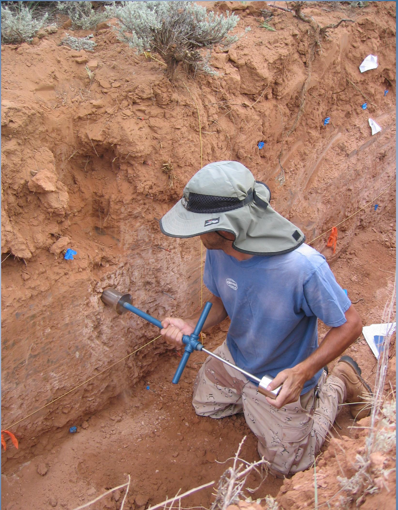
USGS scientist sampling bulk density to characterize soil properties in a backhoe trench dug to investigate soil and stratigraphic controls on boundaries between sagebrush and grasslands.
