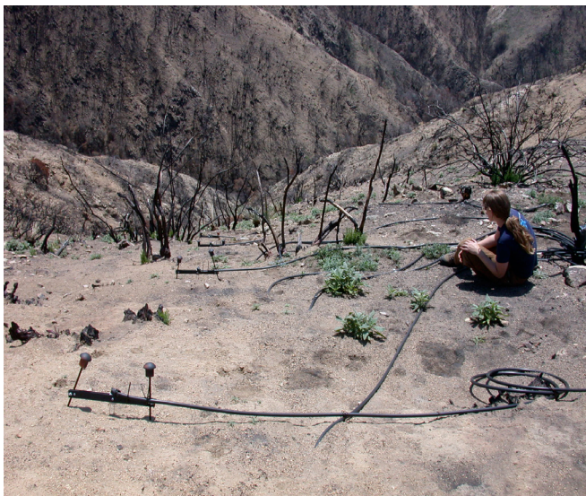
Overland flow detectors on surface of hillslope monitoring location in Day Fire Intensive Research Area.
