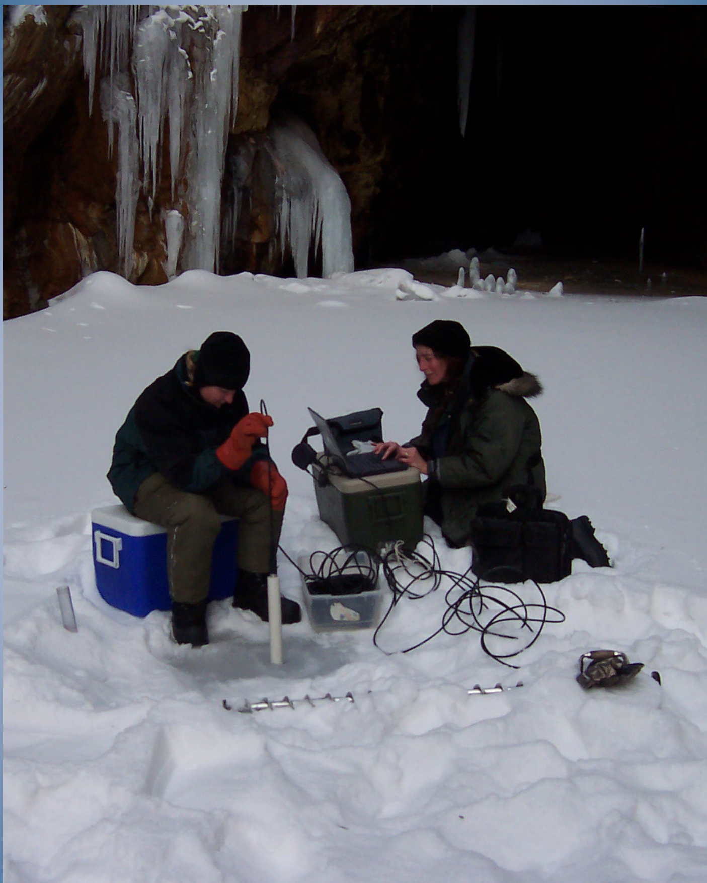
USGS scientists conducting a water column survey of a frozen pit lake at the Elizabeth mine superfund site in Vermont.
