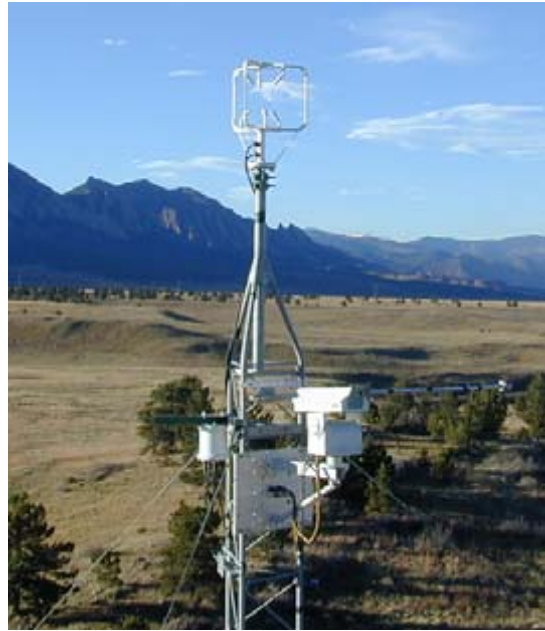
Figure 11. Sonic anemometer mounted on a meteorological tower
