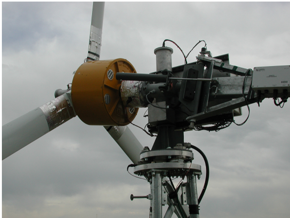
Figure 7. SWRT showing shaft sensor, furl sensor, and tower-leg load cells
