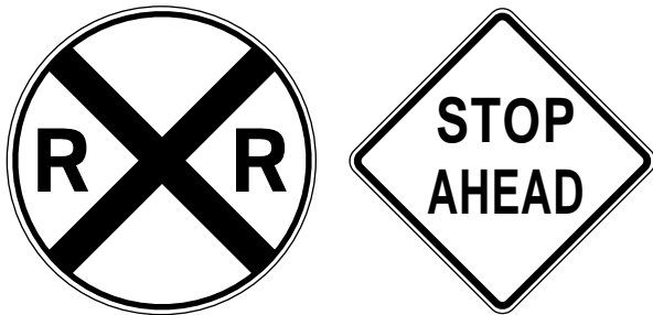
Figure 141: Signs W10-1 and W3-1
