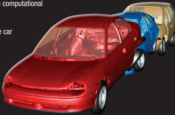
This screen shot of a three-dimensional finite-element model shows a three-car crash. In this type of simulation, separate processors compute the physics of small areas of each car but combine to determine the dynamics of the entire system.
