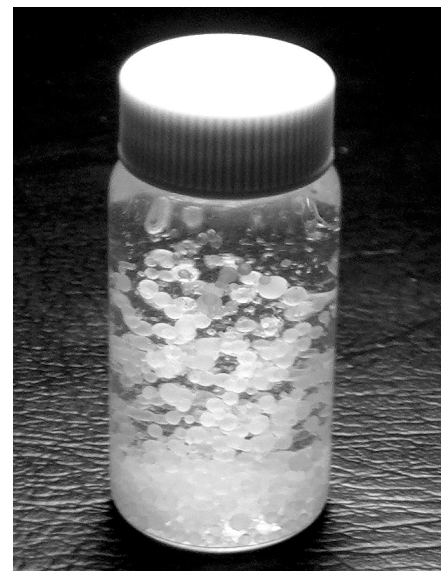
Figure 2: Octoil in water emulsion stabilized with ~10 μm CaCO 3 particles.
