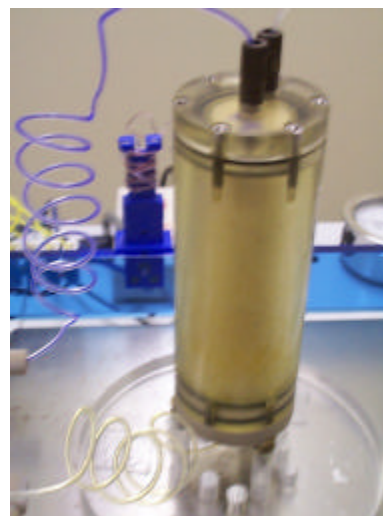
Figure 6. Close Up Photo of PUF Column After 72 h of Injection with \text{Ca}(\text{OH})_2 and \text{CO}_2(\text{g}) . Note very small blue area just under the \text{Ca}(\text{OH})_2 inlet that defines the calcite precipitation front.
