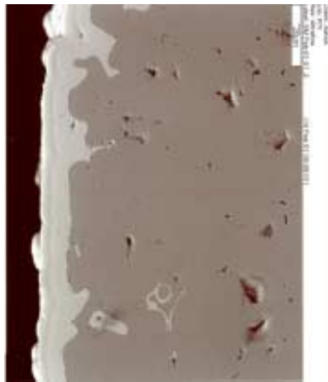
Figure 7. 3-Layer Plating on Porous Stainless Steel Substrate
