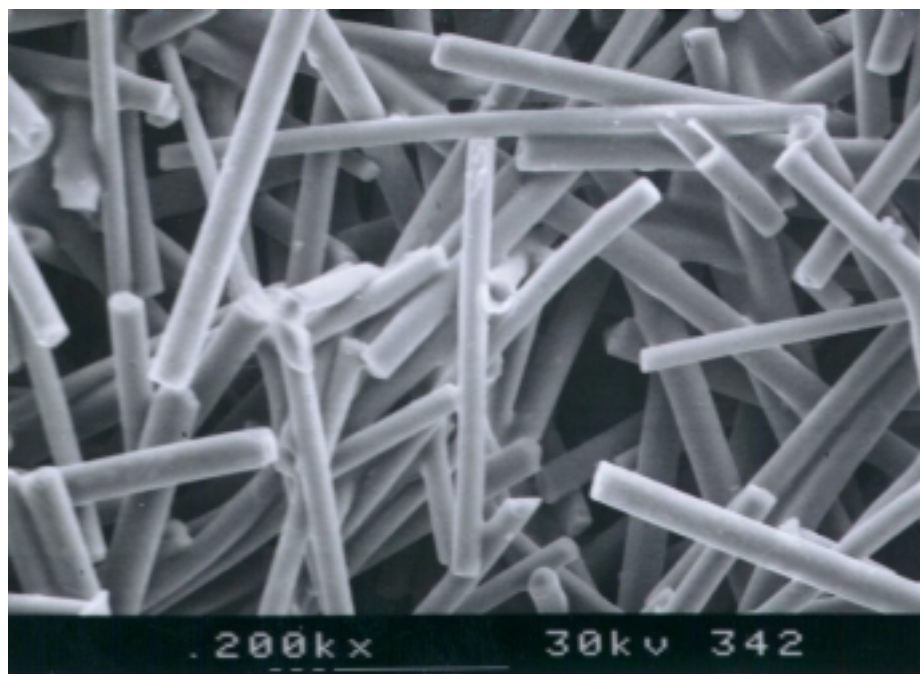
Fig. 1. Micrograph of the CFCMS showing the open structure of the material.
