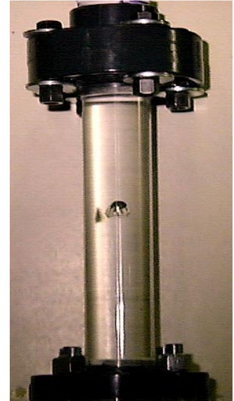
Air bubble stabilized in downward flow of water in low pressure water tunnel
