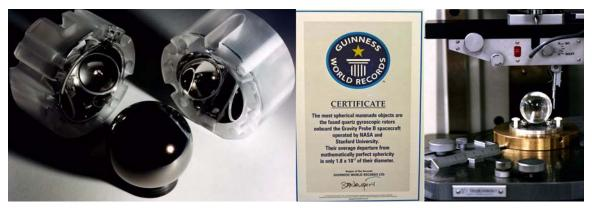
**Figure 1-4.** A GP-B niobium-coated gyro rotor and housing (left), the Guinness Database record for roundness (center), and measuring the sphericity of a gyro rotor (right)
