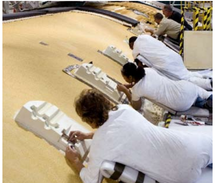
Lockheed Martin technicians at NASA's Michoud Assembly Facility apply ice frost ramps to ET-128.
