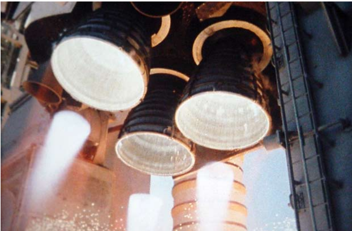
The space shuttle main engine is the world's most sophisticated reusable rocket engine. During a shuttle launch, the shuttle's three engines operate for about eight-and-one-half minutes during liftoff and ascent.
