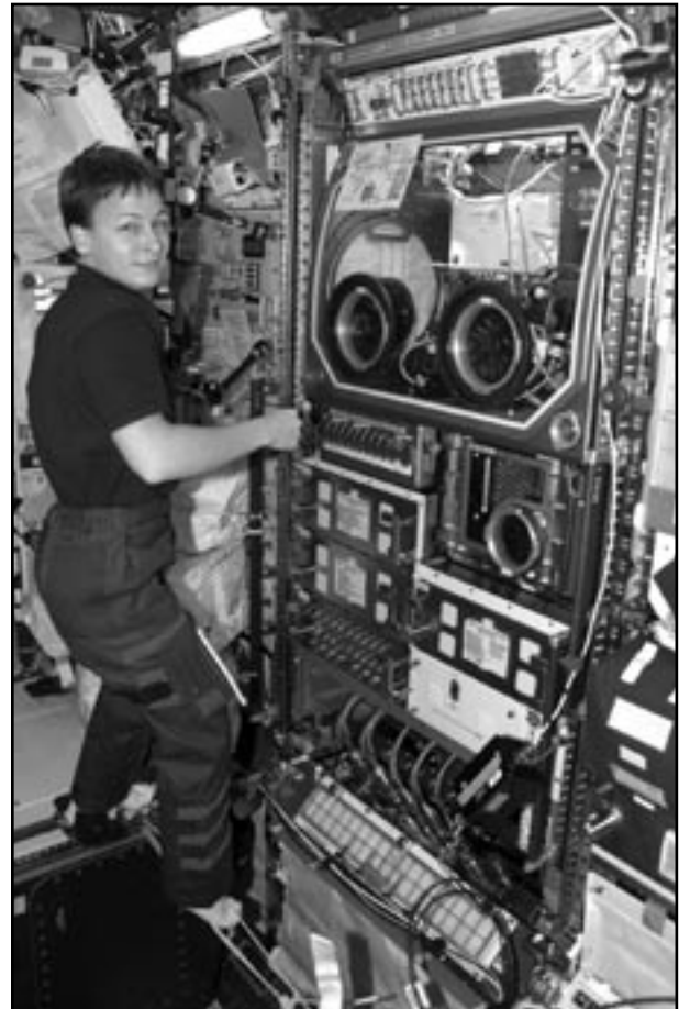
Flight Engineer Peggy Whitson works with the Microgravity Science Glovebox aboard the International Space Station, preparing for a materials experiment to study semiconductor-manufacturing processes.
