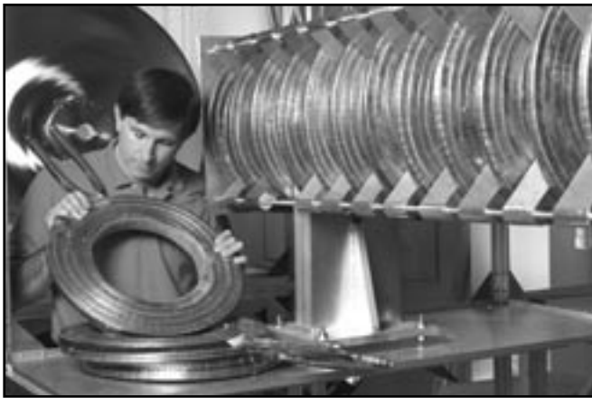
Bill Emrich, a Marshall center researcher, studies components of the gas-dynamic mirror—a magnetic, mirror-based fusion propulsion system now being tested at Marshall's Propulsion Research Center facilities.
