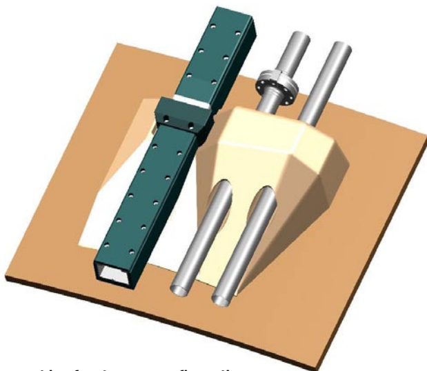
Current ice frost ramp configuration.
