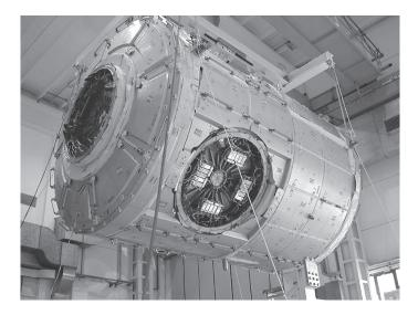
Weighing approximately 30,000 pounds, Node 2 is the second of three connectors between International Space Station modules. International contractor Alenia Spazio built Node 2 at its facility in Torino, Italy. Workers there prepared the Node for shipment to NASA's Kennedy Space Center in Florida on June 1, 2003. Node 2 is more than 20 feet long and 14.5 feet wide.
