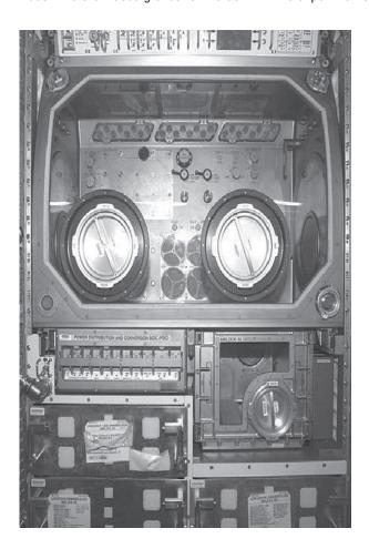
installed and operating inside the Glovebox, providing a barrier against chemicals and gases that might otherwise be potentially hazardous. In keeping with the international flavor of the Space Station program, the Glovebox rack was built by the European Space Agency, but is managed and operated by specialists at the Microgravity Development Laboratory.
