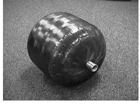
An ultra lightweight composite overwrapped tank, designed and fabricated by Carleton Pressure Technology Division of Westminster, Md., and NASA's Jet Propulsion Laboratory in Pasadena, Calif., during the development phase of the Mars Exploration Rover Program. Research of lightweight in-space propulsion system tank technologies is sponsored by the In-Space Propulsion Technology Project at the Marshall Space Flight Center in Huntsville, Ala.
