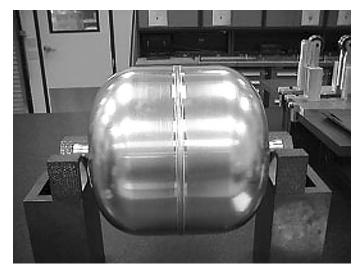
An aluminum liner for ultra-lightweight tank technologies, designed and fabricated by Carleton Pressure Technology Division of Westminster, Md., and NASA's Jet Propulsion Laboratory in Pasadena, Calif., during the development phase of the Mars Exploration Rover Program. Research of lightweight in-space propulsion system tank technologies is sponsored by the In-Space Propulsion Technology Project at the Marshall Space Flight Center in Huntsville, Ala.
