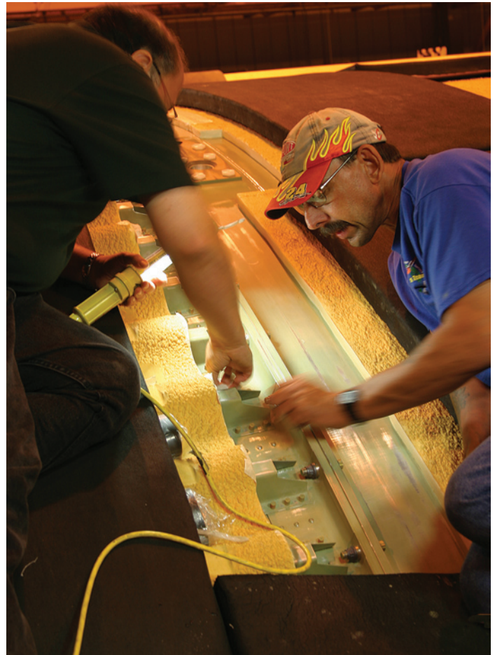
Two NASA technicians inspect the flange that joins the liquid hydrogen tank and intertank on the external tank.
